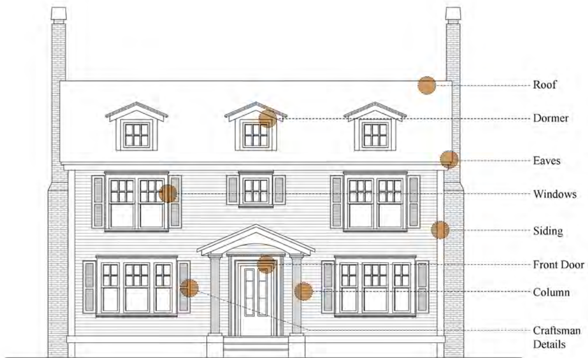
Figure 5.12: Colonial Revival Facade Features
