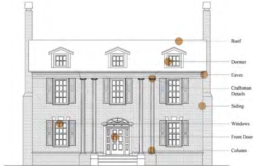
Figure 5.24: Neo-Classical Facade Features
