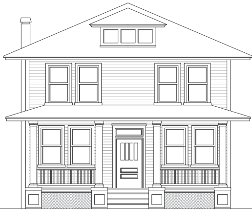
Example: Traditional Four Square Facade
