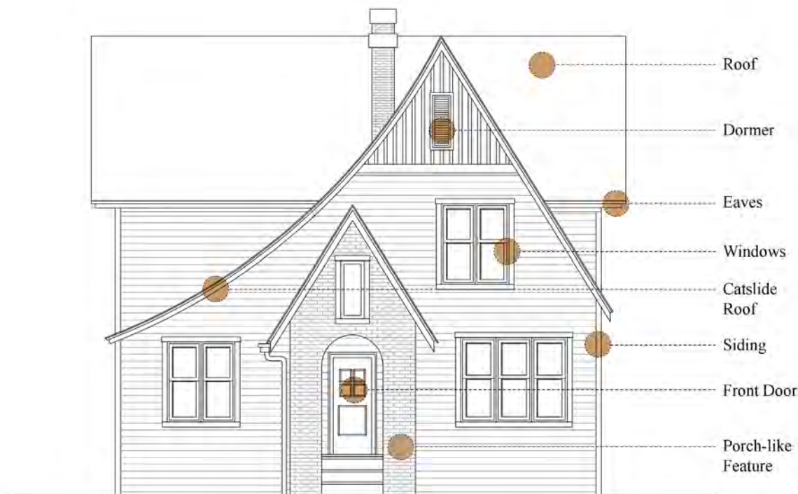
Figure 5.30: Tudor Facade Features
