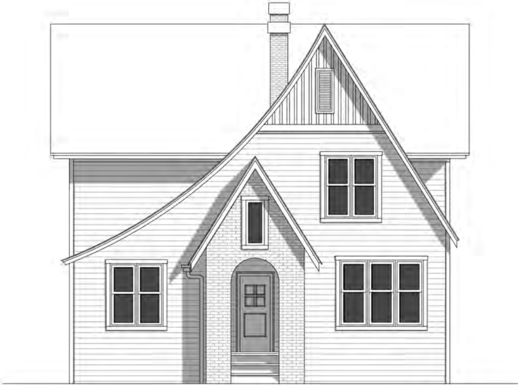
Figure 5.29: Facade Conditions from Tudor House Style
