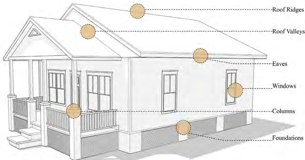
Figure 7.1: Conditions of House Features to be assessed
