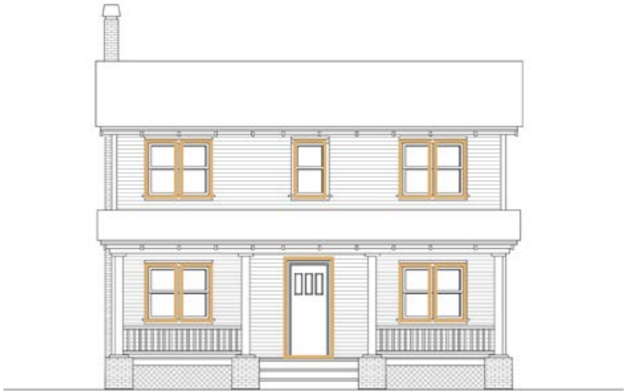
Figure 4.20: Acceptable Window Configurations
