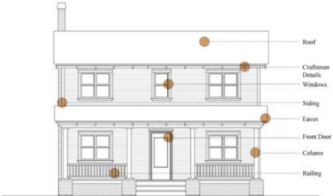
Figure 5.3: Frame Vernacular Facade Features
