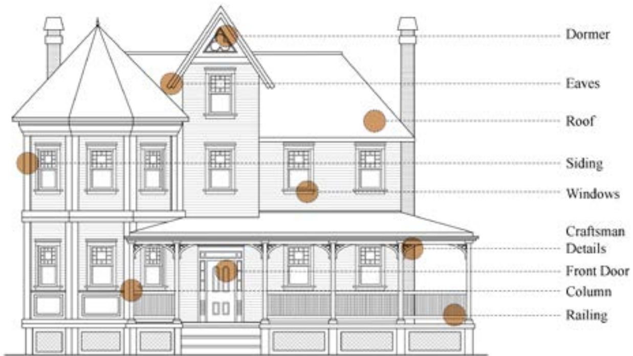
Figure 5.15: Queen Anne Facade Features
