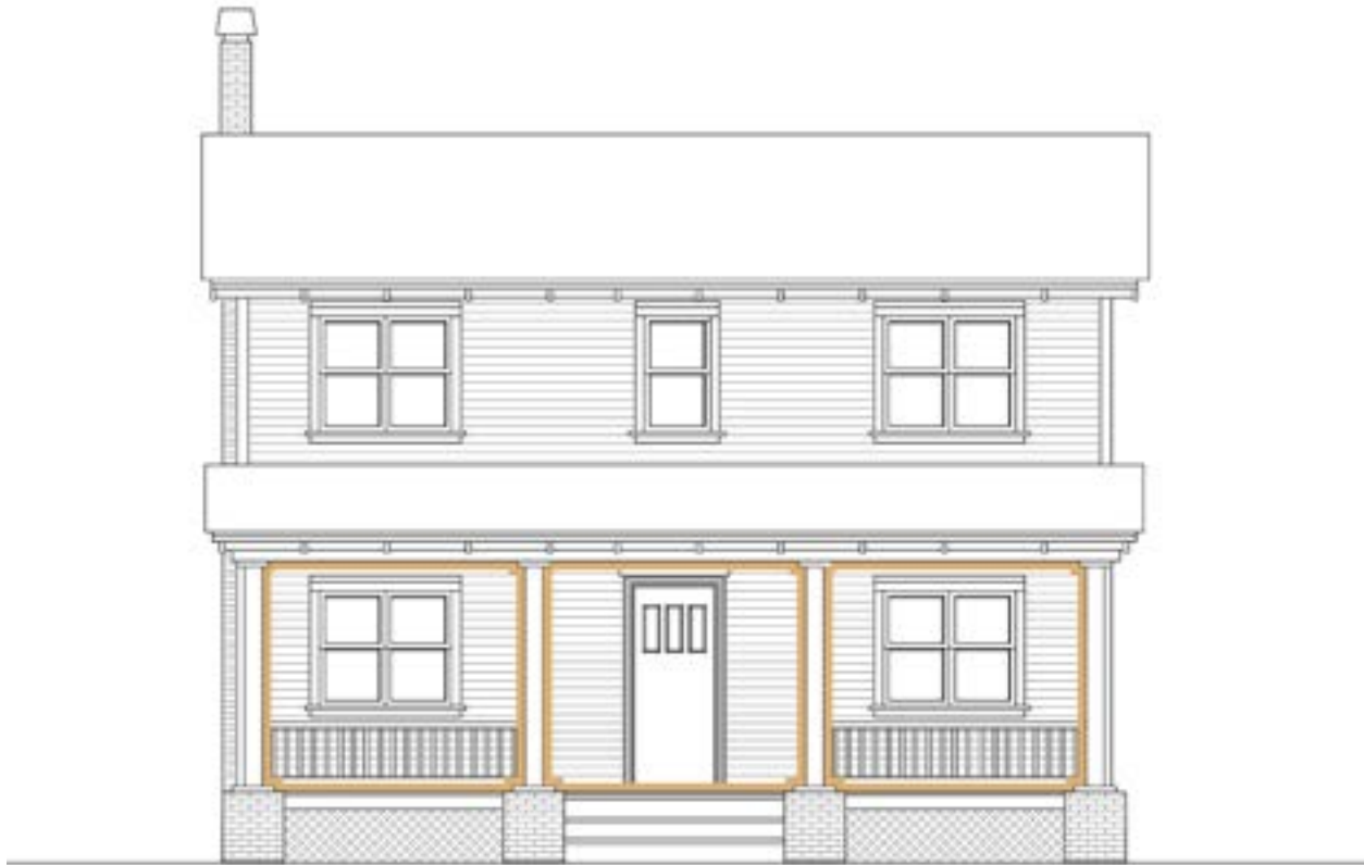
Figure 4.18: Regular Arrangement of Porch Columns and Wall Openings
