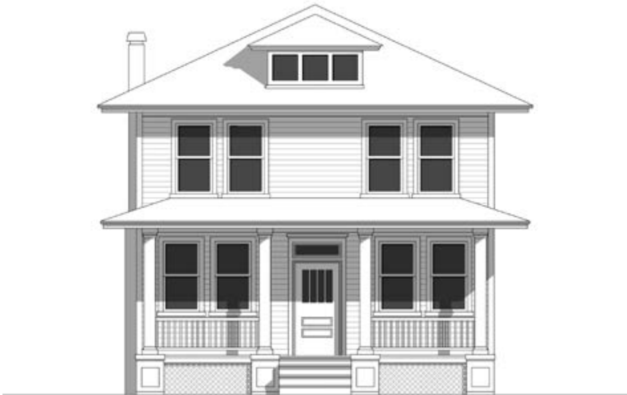
Figure 5.17: Facade Conditions from Four Square House Styles
