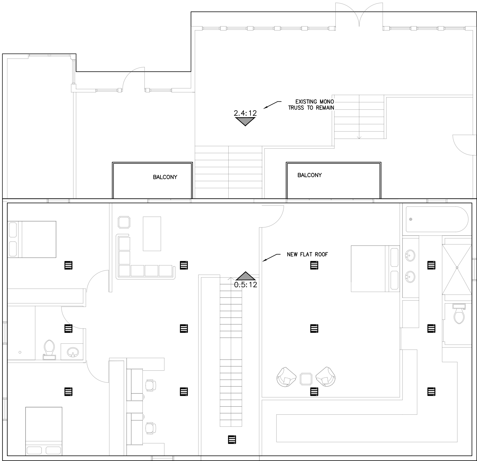
PROPOSED ROOF LAYOUT 1/8"=1'-0"
