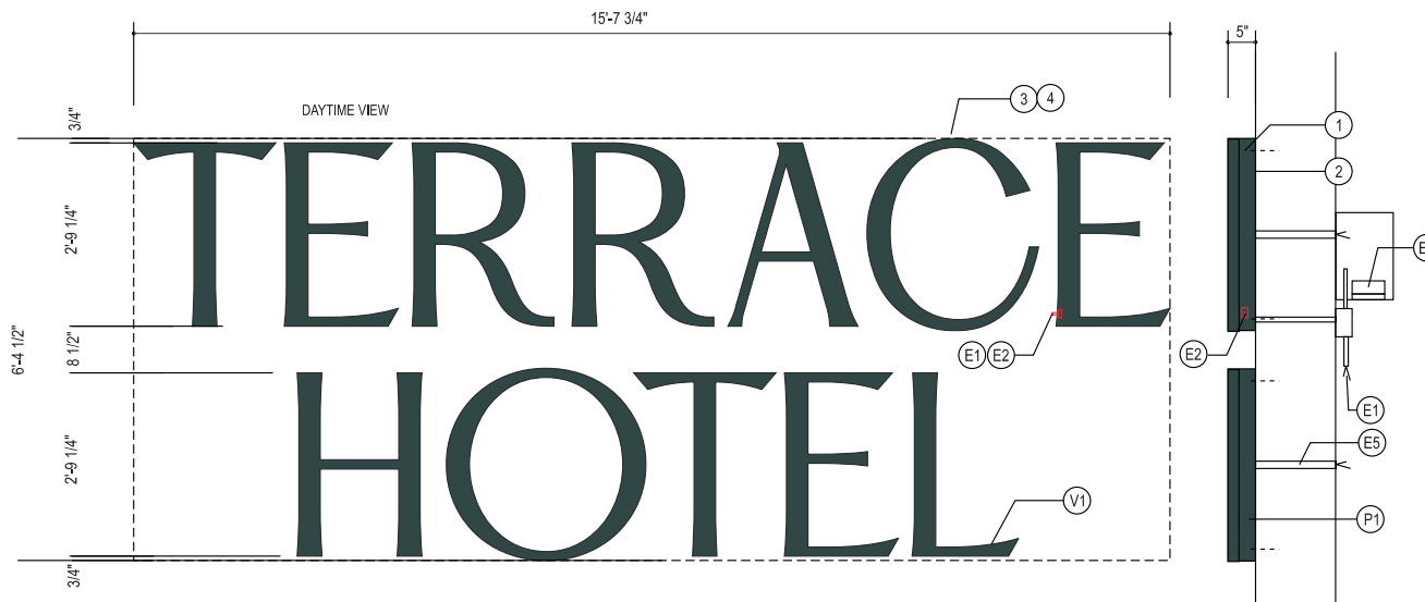
A PARTIAL / FRONT ELEVATION / NORTH 99.710 SQ. FT. Scale: 1/2"=1'-0"
