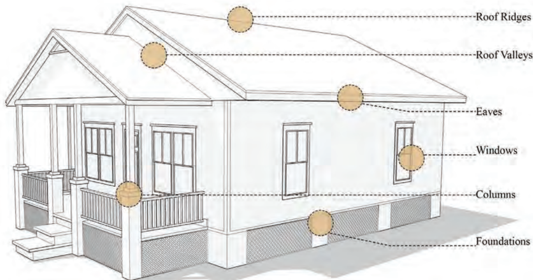
Figure 7.1: Conditions of House Features to be Assessed
