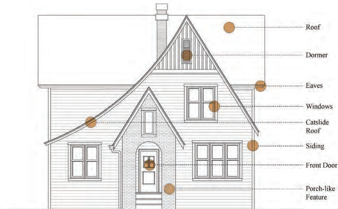
Figure 5.36: Tudor Facade Features
