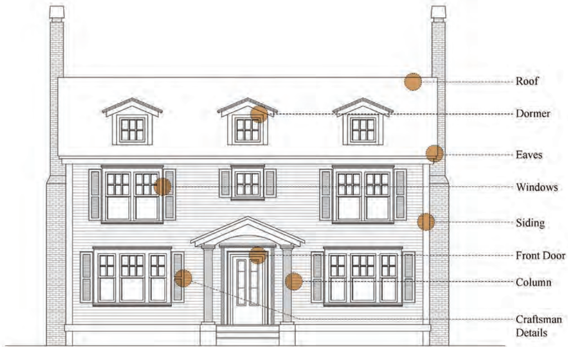
Figure 5.12: Colonial Revival Facade Features
