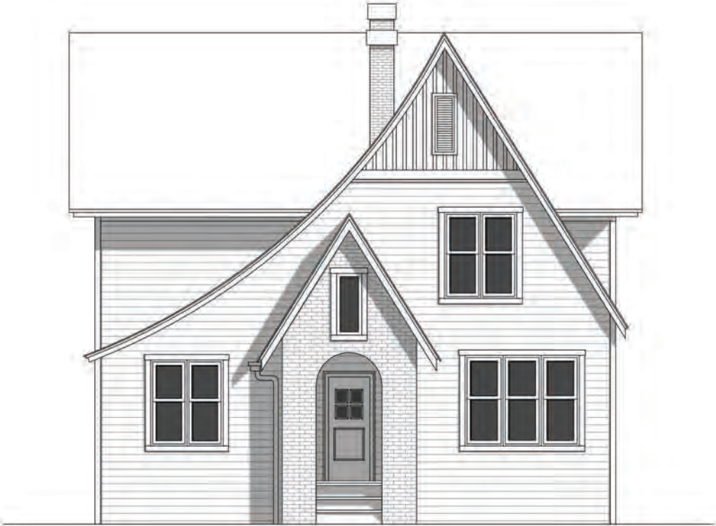
Figure 5.35: Facade Conditions from Tudor House Style
